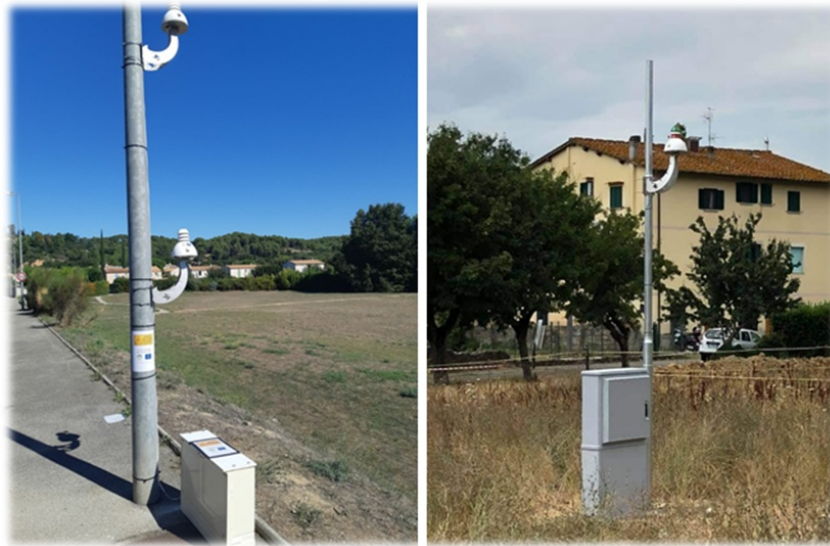
Fig. 4 - Set-up of the air quality and meteorological sensors to measure baseline conditions before tree planting in Aix-en-Provence (left) and Florence (right). The sensors are placed vertically, unsheltered, at 1.8 m and 3.0m above the ground.
