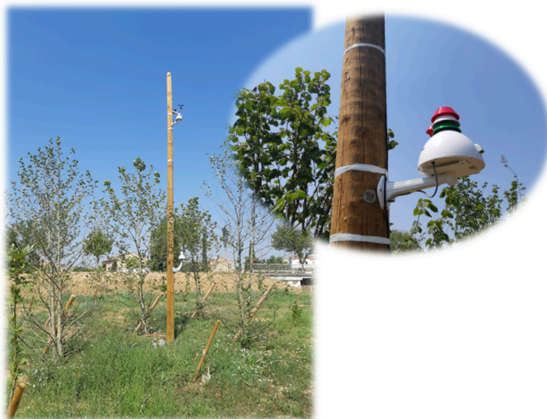
Fig. 1 - Test area in Aix-en-Provence: tree planting in January 2022, 400 fast-growing trees, mix of species, > 3 m tall, equivalent to 1.2ha with AirQino sensors set-up above/below tree canopy, inside/outside test area.
